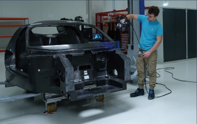
Inspection and Quality Control of Carbon Fiber Monocoque for Hypercars with FreeScan Trak Pro2
