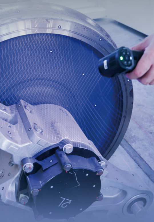
High-speed scan mode with 93 laser lines
