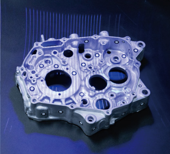
Detailed scan mode with 25 parallel laser lines
