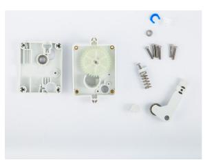
Now it is time to remove the 36 toothed gear. Start by turning the bottom part of the feeder to sideways.
