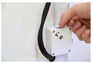
Remove the collet clip, which locks the bowden tube into place.
