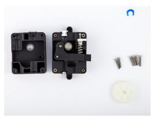
Take the top part of the feeder and carefully put the two pieces back together.
